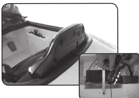
Thermal Circuit Breaker Device
