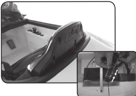
Thermal Circuit Breaker Device
